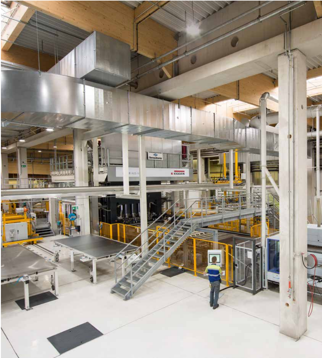
High-tech in practical use: The new short-cycle press that started operation in 2013 in St. Johann in Tirol (AT) is the first of its kind and is used for the lamination of boards with deep surface textures, synchronised pore surfaces on both sides, and for pressing and laminating compact laminate and thin boards.
