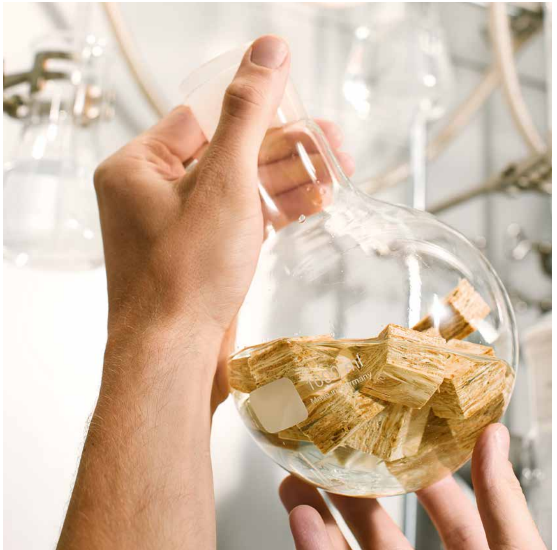
Wood in the laboratory: In the case of the perforator test, the formaldehyde content of wood-based boards is measured by extraction with toluene and subsequent photometric determination.
