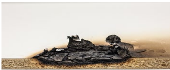
Cross-section Eurodekor Flammex after 30 minutes of burning
