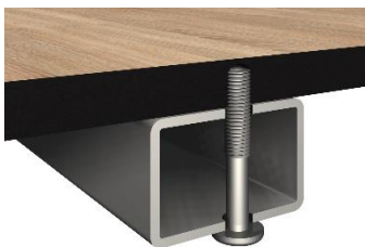
图 40: 防火板桌面板的推荐固定方式 Figure 40: Recommended fastening of the compact tabletop
