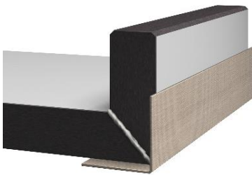
图 18: 折叠竖立件并用胶带固定 Figure 18: Fold up the upstand and secure with adhesive tape
