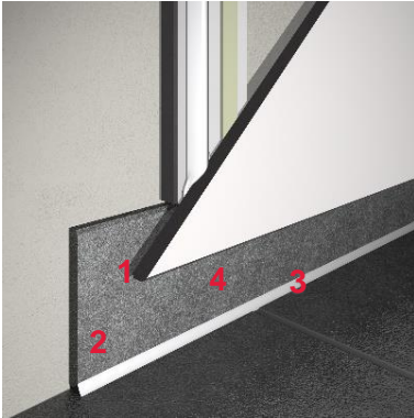
图 31: 墙板底面密封 Figure 31: Bottom closure of the wall cladding
