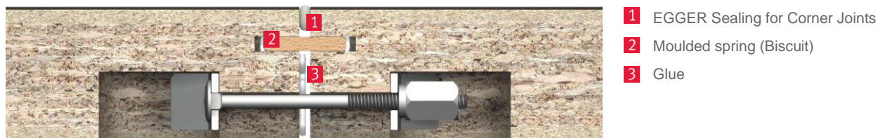
Figure 29: Sealing of worktop corner joint
