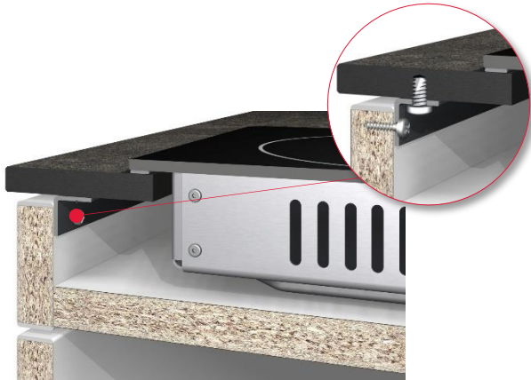
Figure 23: Metal-traverse for cut-outs
