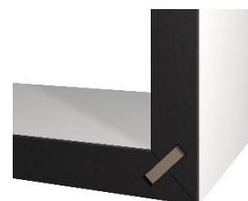
Figure 11: Rainure et languette
