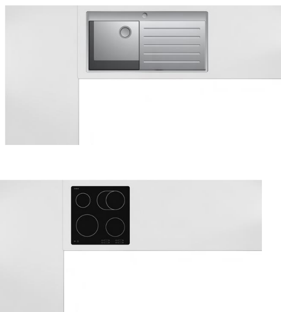
Figure 47: Distance minimale incorrecte
