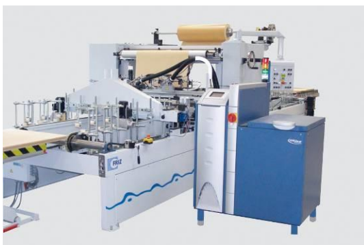
Illustration 3 Machine Type: PROFI FKP 150/1/13/DH/R Application: CPL lamination of doors, including wrapping zone
