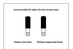
Saw blades with trapezoidal flat tooth are recommended for sawing DecoWall boards with a hand-held circular saw. However, saw blades with hollow roof tooth or hollow trapezoidal tooth are recommended for circular table saws. The finer the teeth, the fewer splinters will occur. You should saw at a reduced feed rate compared to sawing solid wood.
