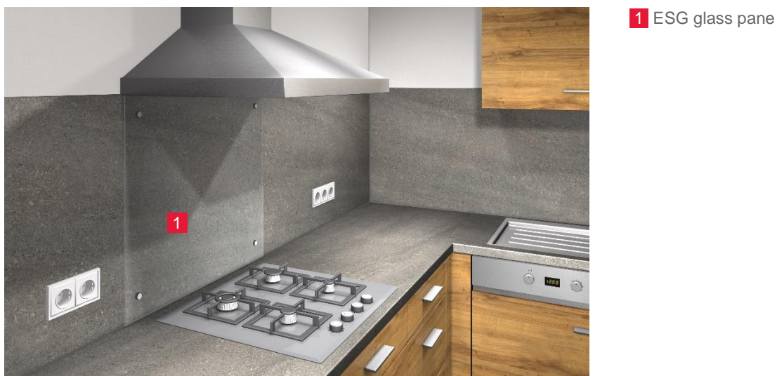
Figure 16: Kitchen situation with gas hob and splashback with ESG glass pane
