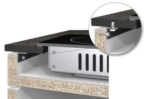
Figure 51: Stabilisation with metal traverse
