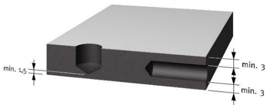
Figure 5: Minimum distances of the drill holes to the edge of the board
