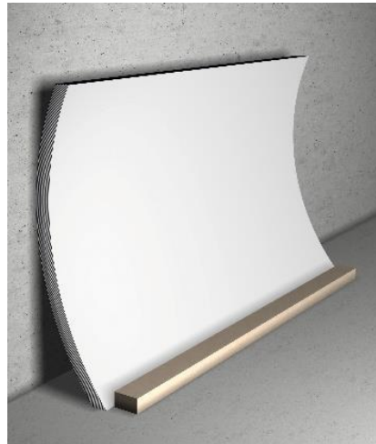
Figure 3: Incorrect storage of compact laminates
