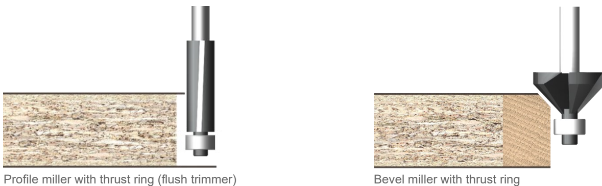
Figure 20: Examples of milling cutters for hand machines
