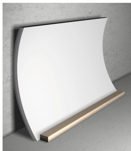
Figure 6: Incorrectly stored laminates
