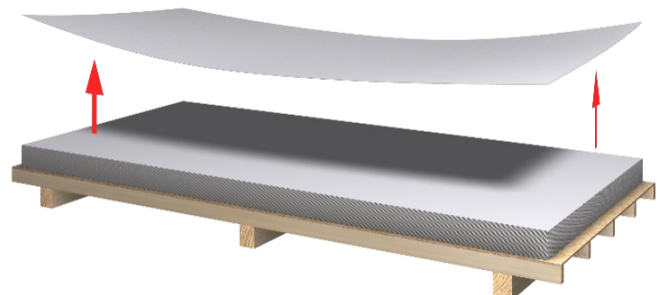
Figure 9: Lifting the laminate
