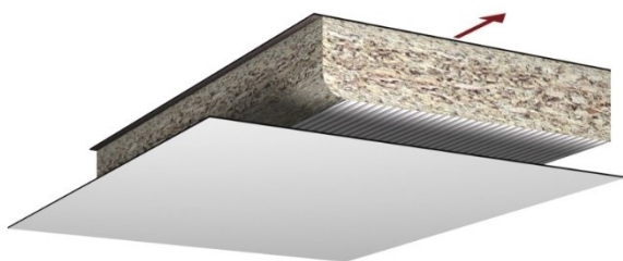
Figure 34: Bonding laminate to core material
