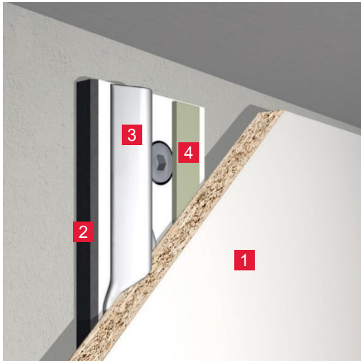
Figure 53: Bonding to a substructure made of compact laminate
