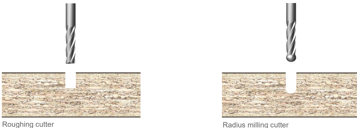
Figure 21: Examples of milling tools on woodworking centers
