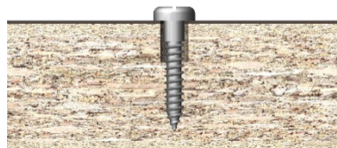
Figure 19: Screw joint with pre-drilling
