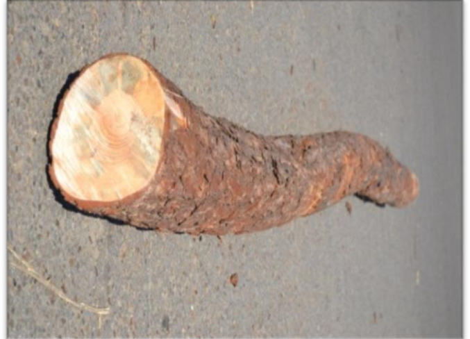
Curbura multipla / Multiple curvature
