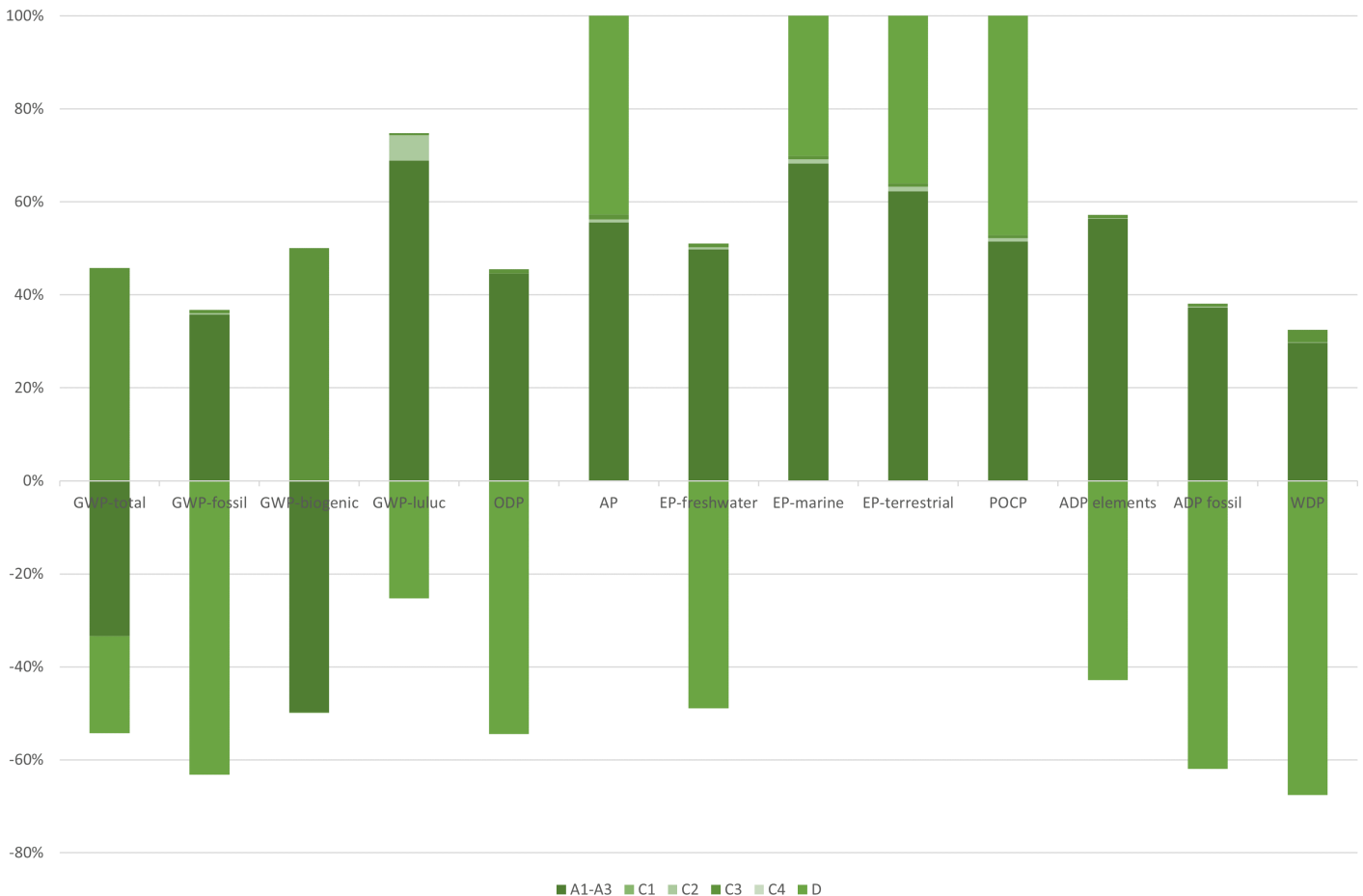
Hot-spot analysis of EGGER PerfectSense lacquered chipboards
