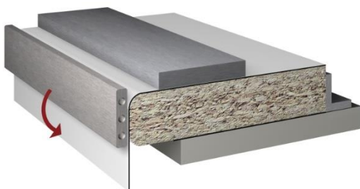
Figure 31: Postforming the laminate
