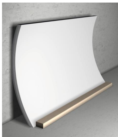
Figure 6: Incorrectly stored laminates
