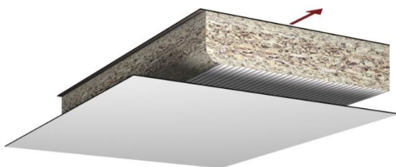
Figure 34: Bonding laminate to core material
