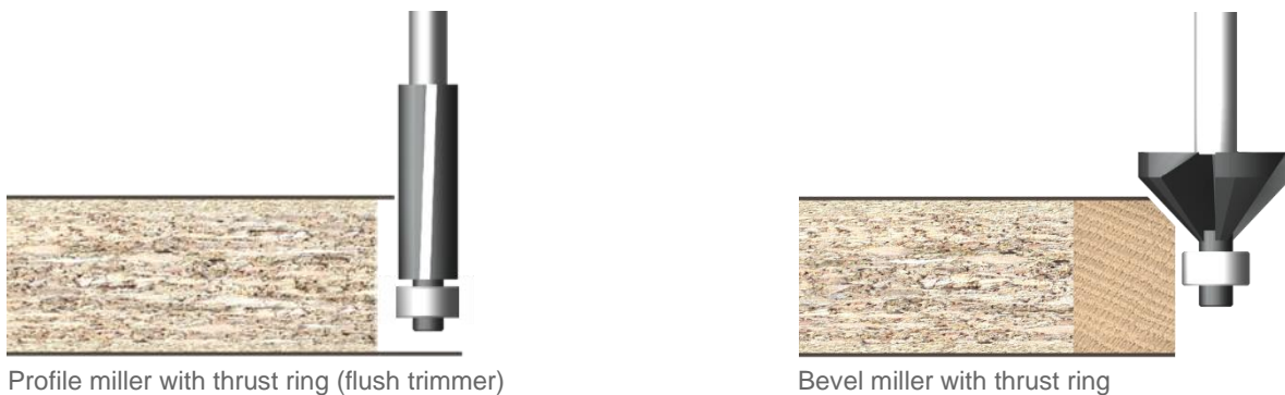
Figure 20: Examples of milling cutters for hand machines
