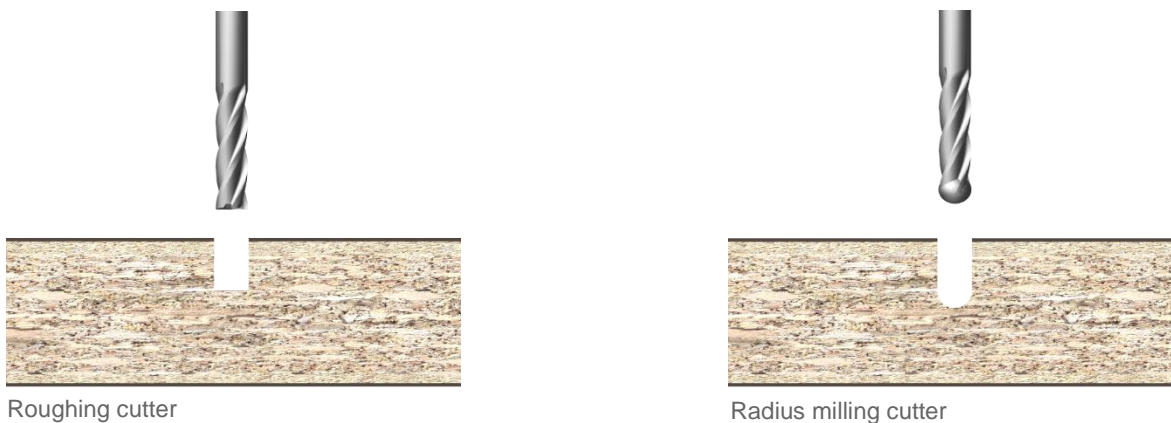
Figure 21: Examples of milling tools on woodworking centres
