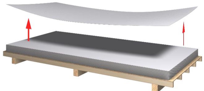
Figure 9: Lifting the laminate
