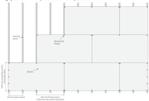
Diagram 8 - typical fixing layout of 1,200 mm wide particleboards on 600 mm joist centres
