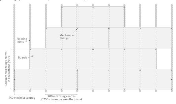
Diagram 6 - typical fixing layout of 600 mm wide particleboards on 600 mm joist centres
