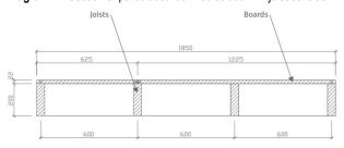
Diagram 5 - typical fixing layout of 600 mm wide particleboards on 450 mm joist centres
