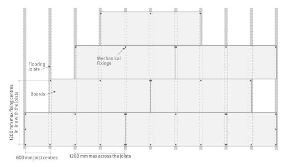
Diagram 7 - typical fixing layout of 1,200 mm wide particleboards on 450 mm joist centres
