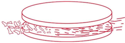
Step 3: Defibering in the refiner
