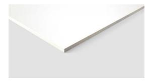
Egger compact laminates white core are compact laminates according to DIN EN 438-9 with a white core based on curable resins. They have a multilayer structure and consist of melamine resin impregnated decorative paper and multiple layers of soda kraft paper impregnated with phenolic resins, which are laminated under high pressure and heat.
