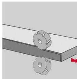
Pre-milling: Pre-mill head at 15 - 20° angle
