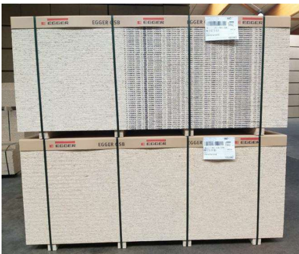
(Image 3): Example for top cardboard cover applied on OSB straight edge packs
