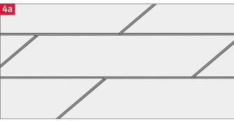
Apply EGGER Joint & Joist Adhesive along the next row of joists and stagger the next row of panels by approximately half a board to form a brick bond laying pattern. Repeat steps (excluding step 2) and note that care should be taken when walking on newly laid boards.
