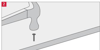
Lay the boards across the joist and fix the first row of boards with only one mechanical fixing (2.5 times the board thickness) per joist along the perimeter edge, minimum 8 mm from the joint edge.
