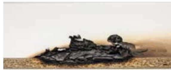
Cross-section Eurodekor Flammex after 30 minutes of burning
