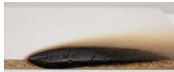
Cross-section Eurodekor after 30 minutes of burning
