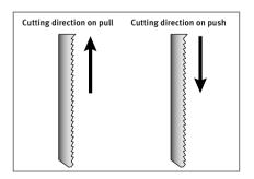
**Attention:** The cutting direction of the saw blade used must be observed. The jigsaws can work on pull (usual case) or on push.
