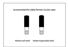
Saw blades with trapezoidal flat tooth are recommended for sawing DecoWall boards with a hand-held circular saw. However, saw blades with hollow roof tooth or hollow trapezoidal tooth are recommended for circular table saws. The finer the teeth, the fewer splinters will occur. You should saw at a reduced feed rate compared to sawing solid wood.
