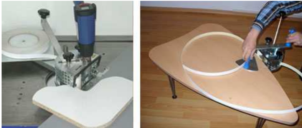
Illustration: Using the "Kantenknirps" edge banding machine www.kantenknirps.de
