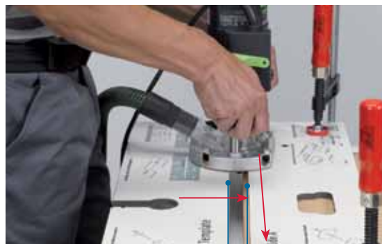
Inset for the guide bush (inside channel) Inset for the guide bush (outside channel)
